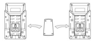
Connecting two expansion modules on a single host phone is shown as below:
