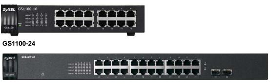
The GS1100-24 has two mini-GBIC ports for uplink connection. Use mini-GBIC transceivers in these slots for connections to backbone Ethernet switches.
