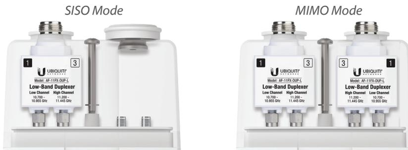
Example of SISO Mode vs MIMO Mode Configuration
