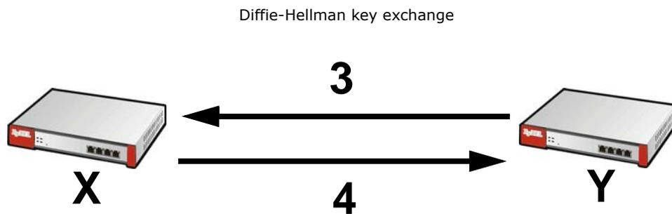
DH public-key cryptography is based on DH key groups. Each key group is a fixed number of bits long. The longer the key, the more secure the encryption, but also the longer it takes to encrypt and decrypt information. For example, DH2 keys (1024 bits) are more secure than DH1 keys (768 bits), but DH2 keys take longer to encrypt and decrypt.
