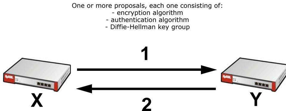
The ZyWALL/USG sends one or more proposals to the remote IPsec router. (In some devices, you can only set up one proposal.) Each proposal consists of an encryption algorithm, authentication algorithm, and DH key group that the ZyWALL/USG wants to use in the IKE SA. The remote IPsec router selects an acceptable proposal and sends the accepted proposal back to the ZyWALL/USG. If the remote IPsec router rejects all of the proposals, the ZyWALL/USG and remote IPsec router cannot establish an IKE SA.
