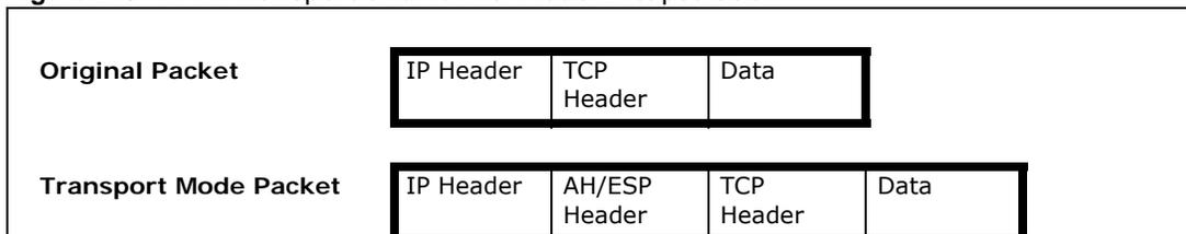
**Figure 270** VPN: Transport and Tunnel Mode Encapsulation
