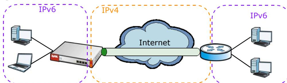
In the ZyWALL/USG, you must also manually configure a policy route for an IPv6-in-IPv4 tunnel to make the tunnel work.
