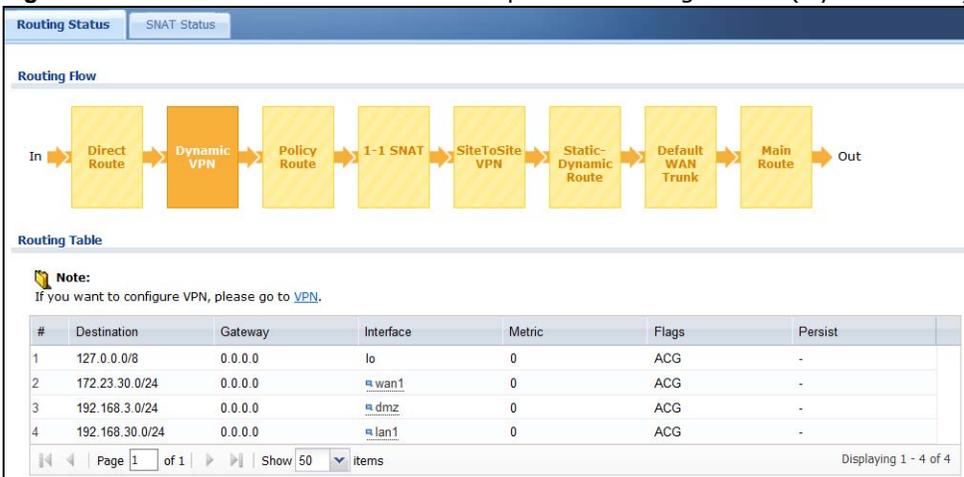
Figure 534 Maintenance > Packet Flow Explore > Routing Status (Static-Dynamic Route)
