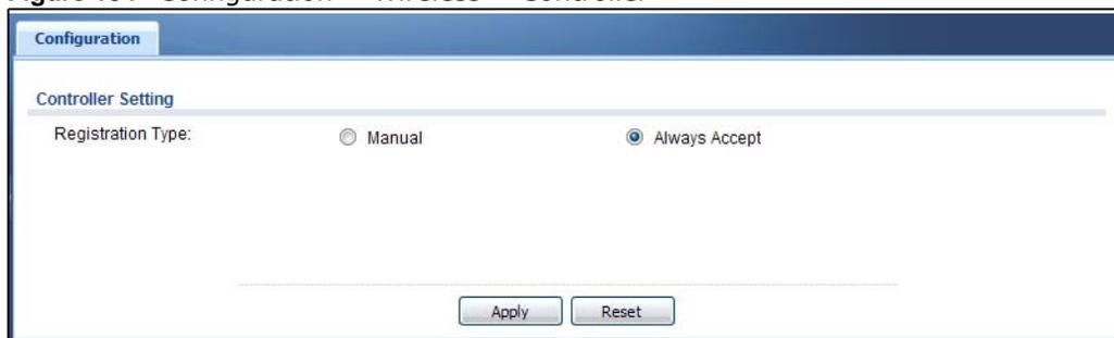
The screenshot displays the 'Configuration > Wireless > Controller' screen. At the top, there is a 'Configuration' tab. Below it, the 'Controller Setting' section is visible. Under 'Registration Type', there are two radio button options: 'Manual' (unselected) and 'Always Accept' (selected). At the bottom of the screen, there are two buttons: 'Apply' and 'Reset'.
