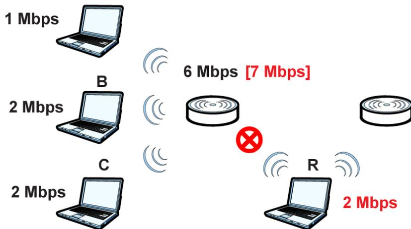
Connections are kicked based on either **idle timeout** or **signal strength**. The ZyWALL/USG first looks to see which devices have been idle the longest, then starts kicking them in order of highest idle time. If no connections are idle, the next criteria the ZyWALL/USG analyzes is signal strength. Devices with the weakest signal strength are kicked first.
