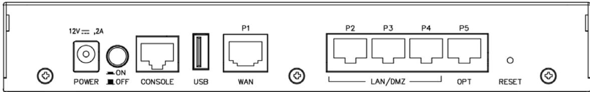
**Figure 39** USG60 / USG60W Rear Panel
