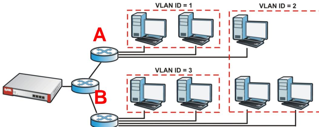
Each VLAN is a separate network with separate IP addresses, subnet masks, and gateways. Each VLAN also has a unique identification number (ID). The ID is a 12-bit value that is stored in the MAC header. The VLANs are connected to switches, and the switches are connected to the router. (If one switch has enough connections for the entire network, the network does not need switches **A** and **B**.)
