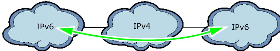
On the ZyWALL/USG, you can either set up a manual IPv6-in-IPv4 tunnel or an automatic 6to4 tunnel. The following describes each method:
