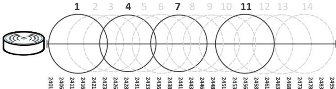
However, some regions require the use of other channels and often use a safety scheme with the following four channels: 1, 4, 7 and 11. While they are situated sufficiently close to both each other and the three so-called "safe" channels (1,6 and 11) that interference becomes inevitable, the severity of it is dependent upon other factors: proximity to the affected AP, signal strength, activity, and so on.
