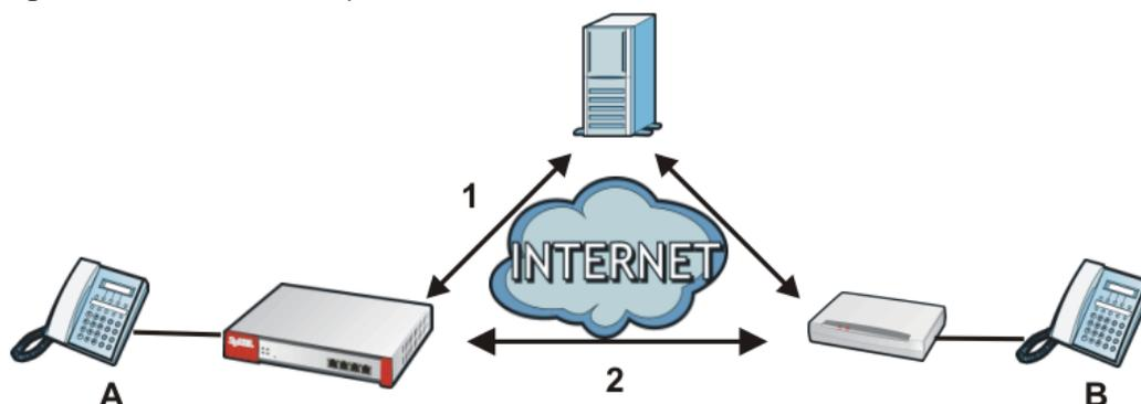
The ALG feature is only needed for traffic that goes through the ZyWALL/USG's NAT.
