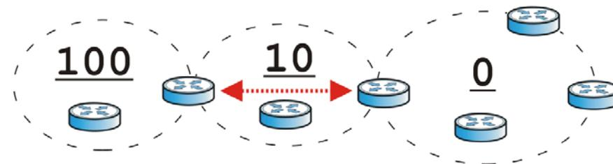
In this example, area 100 does not have a direct connection to the backbone. As a result, you should set up a virtual link on both ABR in area 10. The virtual link becomes the connection between area 100 and the backbone.
