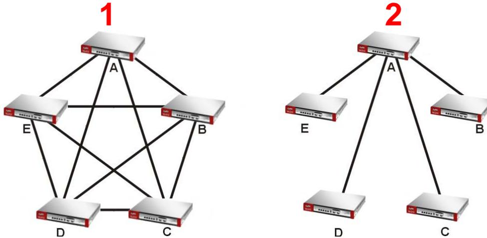
In a fully-meshed VPN topology (1 in the figure), there is a VPN connection between every pair of routers. In a hub-and-spoke VPN topology (2 in the figure), there is a VPN connection between each spoke router (B, C, D, and E) and the hub router (A), which uses the VPN concentrator. The VPN concentrator routes VPN traffic between the spoke routers and itself.
