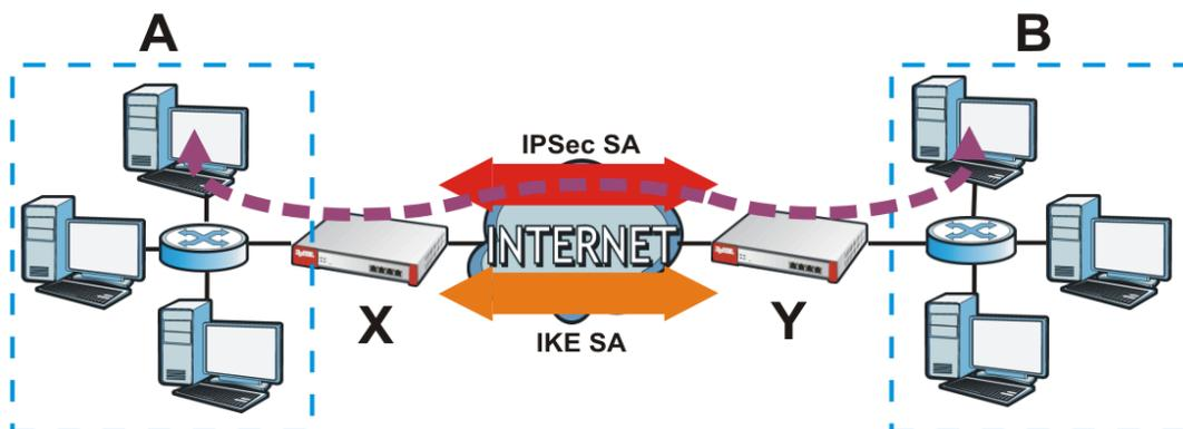
In this example, a computer in network **A** is exchanging data with a computer in network **B**. Inside networks **A** and **B**, the data is transmitted the same way data is normally transmitted in the networks. Between routers **X** and **Y**, the data is protected by tunneling, encryption, authentication, and other security features of the IPsec SA. The IPsec SA is secure because routers **X** and **Y** established the IKE SA first.
