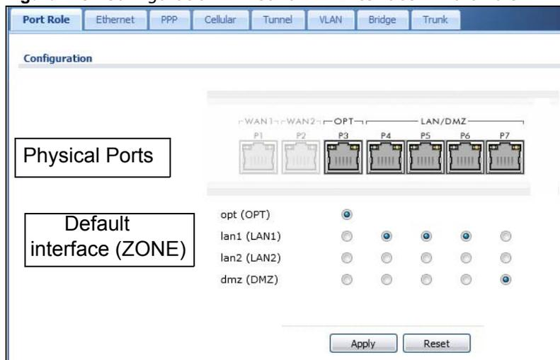
The physical Ethernet ports are shown at the top and the Ethernet interfaces and zones are shown at the bottom of the screen. Use the radio buttons to select for which interface (network) you want to use each physical port. For example, select a port's LAN radio button to use the port as part of the LAN interface. The port will use the ZyWALL/USG's LAN IP address and MAC address.
