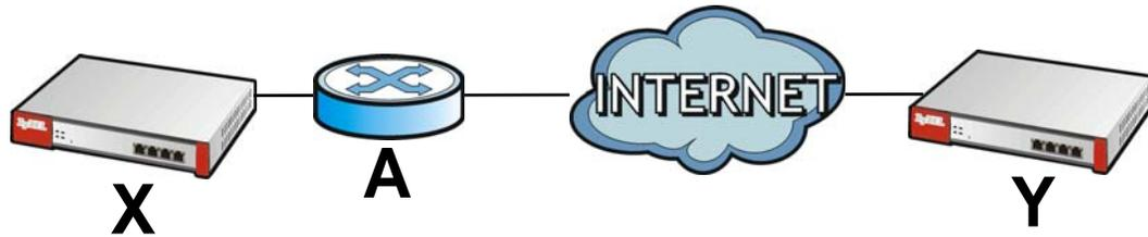
Most routers like router **A** now have an IPSec pass-thru feature. This feature helps router **A** recognize VPN packets and route them appropriately. If router **A** has this feature, router **X** and router **Y** can establish a VPN tunnel as long as the active protocol is ESP. (See [Active Protocol on page 407](#) for more information about active protocols.)
