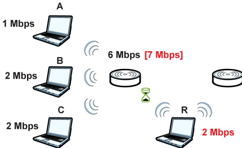
The second response your AP can take is to kick the connections that are pushing it over its balanced bandwidth allotment.
