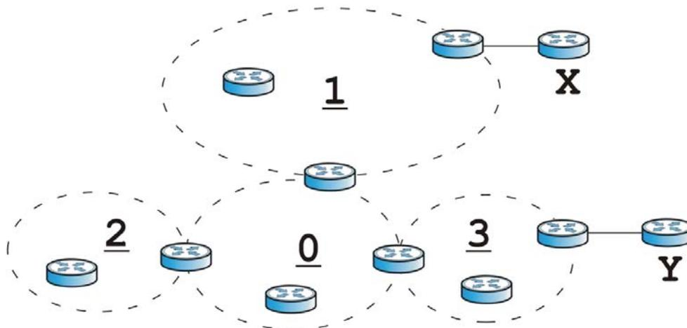
This OSPF AS consists of four areas, areas 0-3. Area 0 is always the backbone. In this example, areas 1, 2, and 3 are all connected to it. Area 1 is a normal area. It has routing information about the OSPF AS and networks X and Y. Area 2 is a stub area. It has routing information about the OSPF AS, but it depends on a default route to send information to networks X and Y. Area 3 is a NSSA. It has routing information about the OSPF AS and network Y but not about network X.
