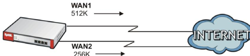
The outbound bandwidth utilization is used as the load balancing index. In this example, the measured (current) outbound throughput of WAN 1 is 412K and WAN 2 is 198K. The ZyWALL/USG calculates the load balancing index as shown in the table below.
