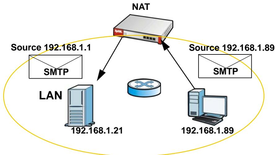
The LAN SMTP server replies to the ZyWALL/USG's LAN IP address and the ZyWALL/USG changes the source address to 1.1.1.1 before sending it to the LAN user. The return traffic's source matches the original destination address (1.1.1.1). If the SMTP server replied directly to the LAN user without the traffic going through NAT, the source would not match the original destination address which would cause the LAN user's computer to shut down the session.
