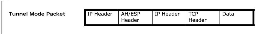
In tunnel mode, the ZyWALL/USG uses the active protocol to encapsulate the entire IP packet. As a result, there are two IP headers:
