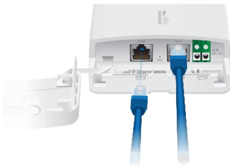
2. Configure the Ethernet adapter on your computer with a static IP address on the 192.168.1.x subnet.
