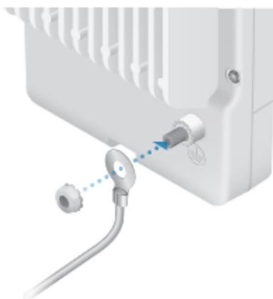
3. At the installation site, secure the other end of the ground wire to a grounded mast, pole, tower, or grounding bar.
