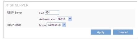
To utilize RTSP authentication, you must first set a password for the camera. RTSP (Real-Time Streaming Protocol) controls the delivery of streaming media. By default the port number is 554.
