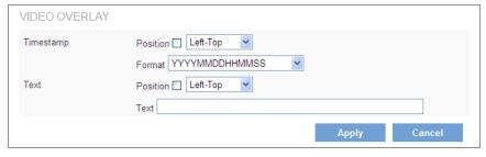
**Timestamp** - To display the date and time on the screen during live view, check the Position check box to enable the timestamp function and select the display position from the drop-down menu.
