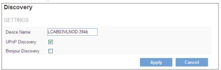
**UPnP Discovery** - Universal Plug and Play (UPnP) simplifies the process of adding a camera to a local area network. Once connected to a LAN, the camera will automatically appear on the intranet.
