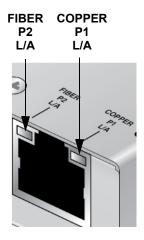
Figure 2. Port LEDs
