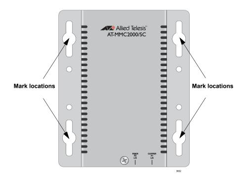
Figure 20. Marking the Screw Hole Locations
