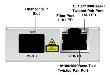
Figure 13. AT-MMC2000/SP Front Panel
