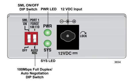
Figure 14. Media Converter Back Panel
