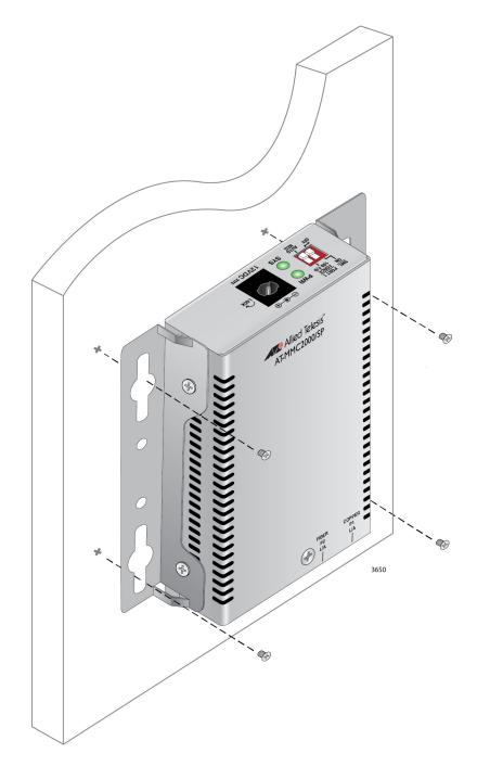
Figure 21. Securing the Media Converter to the Wall
