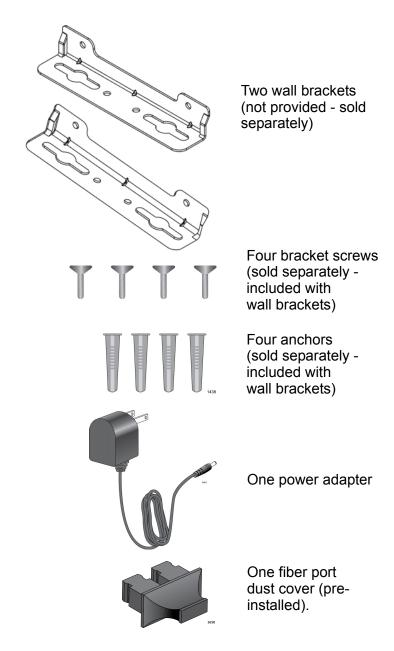
Figure 15. AT-MMC2000/SC and AT-MMC200/SC Shipping Package Contents
