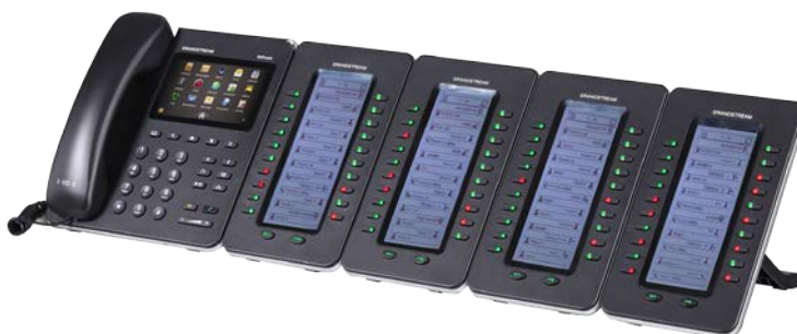
Figure 1: GXP2200EXT 4-Module Front View
