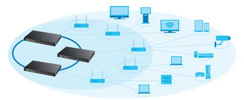
Carrier Ethernet technology employed in the Zyxel MGS3750-28F 24-port GbE L2 Switch with four 10G SFP+ Uplink refers to the utilization of highbandwidth Ethernet technology in Internet access as well as in government, business and academic LAN communications. Carrier Ethernet employs hardware and software to improve connectivity, along with maintenance
