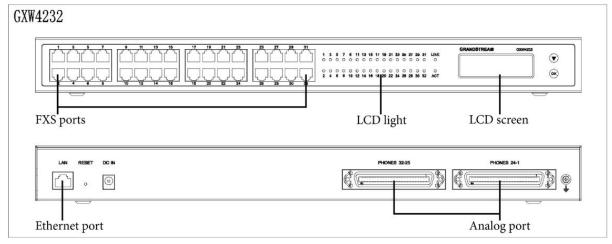
FIGURE 1: DIAGRAM OF GXW4216/24/32 PANEL
