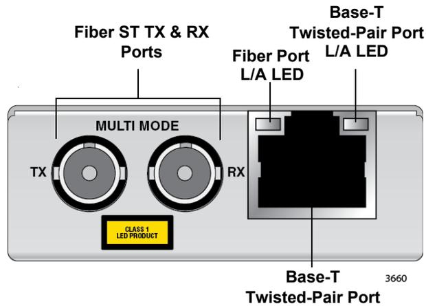
Figure 11. AT-MMC2000/ST and AT-MMC200/ST Front Panel
