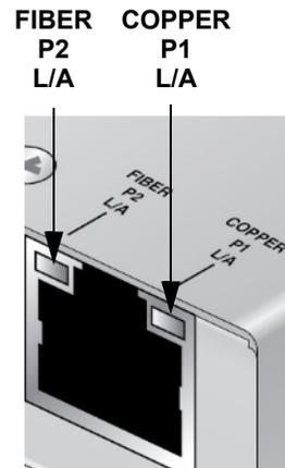
Figure 2. Port LEDs
