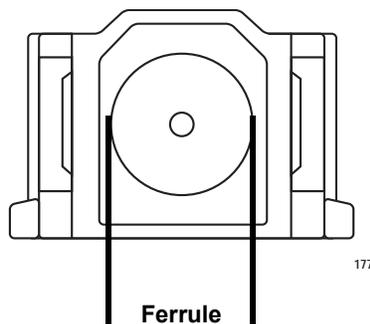
Figure 27. Ferrule in an SC Connector Plug
