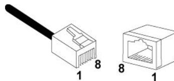
Figure 26. RJ45 Connector and Port Pin Layout
