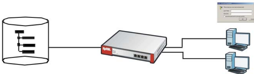
Figure 540 Example: Directory Service Client and Server
