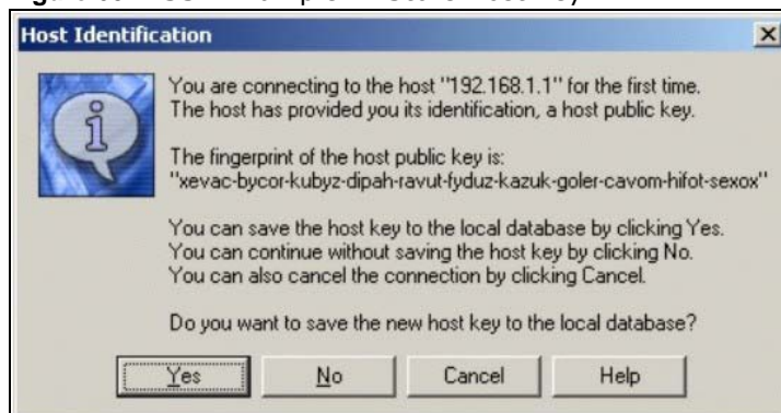
Figure 607 SSH Example 1: Store Host Key
