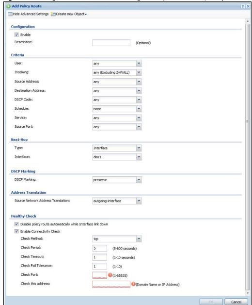
Figure 182 Configuration > Network > Routing > Policy Route > Add/Edit (IPv4 Configuration)
