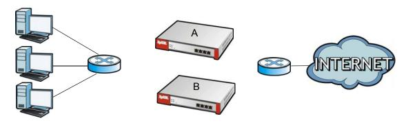
2 Configure the bridge interface on the master ZyWALL/USG, set the bridge interface as a monitored interface, and activate device HA.
