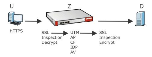
Note: Anti-Spam cannot be applied to traffic decrypted by SSL Inspection.
