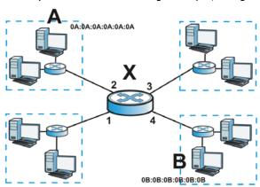
When the bridge receives a packet, the bridge records the source MAC address and the port on which it was received in a table. It also looks up the destination MAC address in the table. If the bridge knows on which port the destination MAC address is located, it sends the packet to that port. If the destination MAC address is not in the table, the bridge broadcasts the packet on every port (except the one on which it was received).
