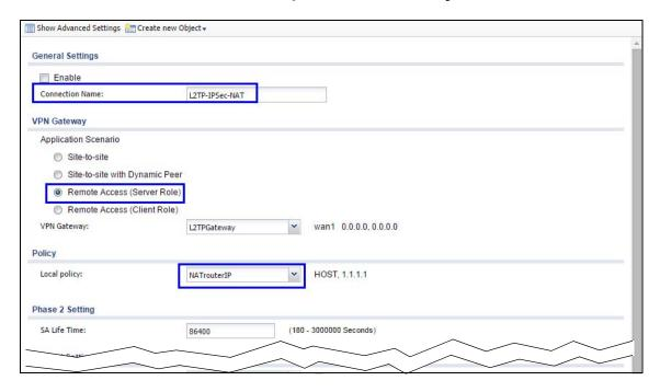
5 Go to Configuration > VPN > L2TP VPN and select the VPN Connection just configured.
