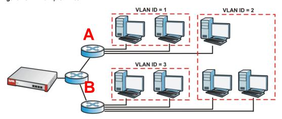
Each VLAN is a separate network with separate IP addresses, subnet masks, and gateways. Each VLAN also has a unique identification number (ID). The ID is a 12-bit value that is stored in the MAC header. The VLANs are connected to switches, and the switches are connected to the router. (If one switch has enough connections for the entire network, the network does not need switches A and B.)
