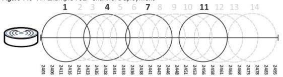
However, some regions require the use of other channels and often use a safety scheme with the following four channels: 1, 4, 7 and 11. While they are situated sufficiently close to both each other and the three so-called "safe" channels (1,6 and 11) that interference becomes inevitable, the severity of it is dependent upon other factors: proximity to the affected AP, signal strength, activity, and so on.
