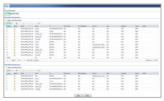
Configure the fields as shown in the following screen. Configure the source and destination addresses according to the SSO web authrntication traffic in your network.
