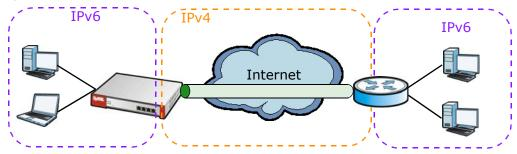
In the ZyWALL/USG, you must also manually configure a policy route for an IPv6-in-IPv4 tunnel to make the tunnel work.
