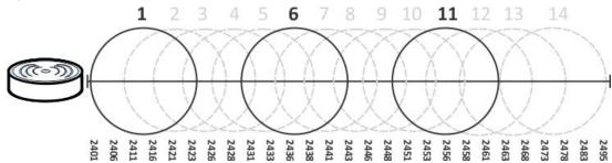
Three channels are situated in such a way as to create almost no interference with one another if used exclusively: 1, 6 and 11. When an AP broadcasts on any of these three channels, it should not interfere with neighboring APs as long as they are also limited to same trio.
