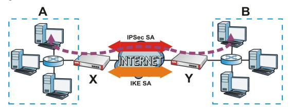
In this example, a computer in network **A** is exchanging data with a computer in network **B**. Inside networks **A** and **B**, the data is transmitted the same way data is normally transmitted in the networks. Between routers **X** and **Y**, the data is protected by tunneling, encryption, authentication, and other security features of the IPSec SA. The IPSec SA is secure because routers **X** and **Y** established the IKE SA first.
