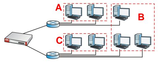
In this example, there are two physical networks and three departments **A**, **B**, and **C**. The physical networks are connected to hubs, and the hubs are connected to the router.
