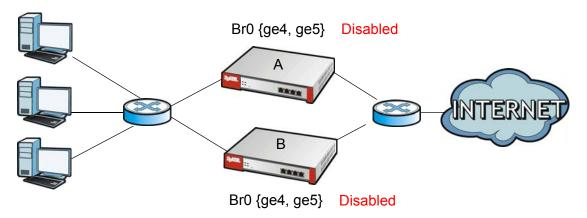
3 Enable the bridge interface on the master ZyWALL/USG and then on the backup ZyWALL/USG.
