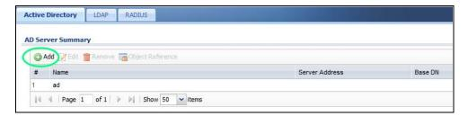
The default AD server port is 389. If you change this, make sure you make the same changes on the SSO. Configure the **Base DN** exactly the same as on the Domain Controller and SSO. **Bind DN** is a user name and password that allows the ZyWALL/USG to join the domain with administrative privileges. It is a required field.
