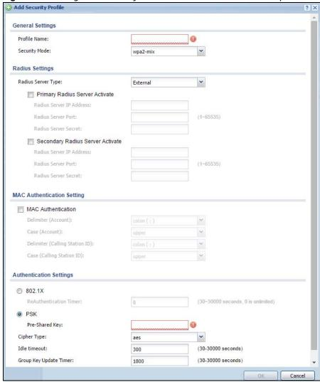
Table 249 Configuration > Object > AP Profile > SSID > Security Profile > Add/Edit Security Profile
