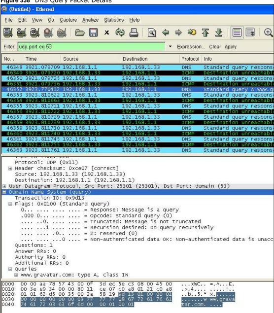
From the details about DNS query you see that the protocol is UDP and the port is 53. The type of DNS packet is standard query and the Flag is 0x0100 with an offset of 2. Therefore enter |010| as the first pattern.
