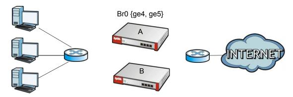
Configure the bridge interface on the backup ZyWALL/USG, set the bridge interface as a monitored interface, and activate device HA.
