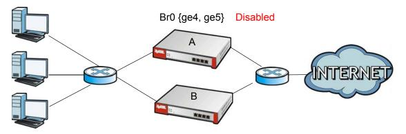
2 Configure a corresponding disabled bridge interface on the backup ZyWALL/USG. Then set the bridge interface as a monitored interface, and activate device HA.
