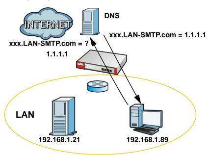
The LAN user's computer then sends traffic to IP address 1.1.1.1. NAT loopback uses the IP address of the ZyWALL/USG's LAN interface (192.168.1.1) as the source address of the traffic going from the LAN users to the LAN SMTP server.
